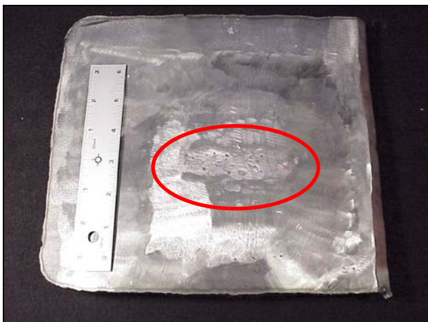
Photo 1: The vessel sample, as received. The pitted area is encircled by the red line.
