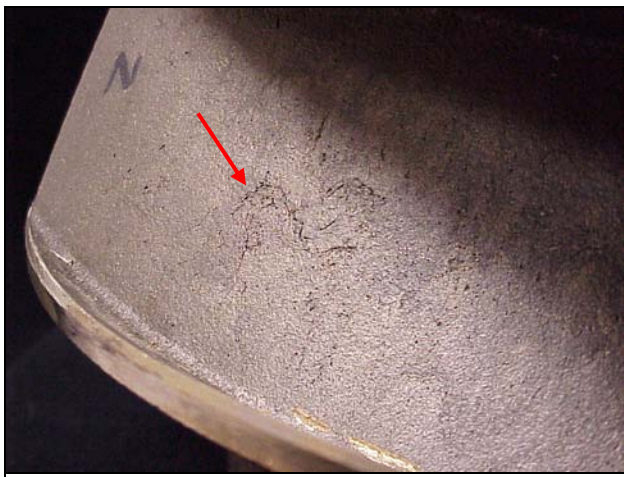
Photo 3: View of defects on vane #2 of Casting #1. .
