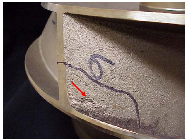
Photo 4: View of defects on vane #6 of Casting #3.
