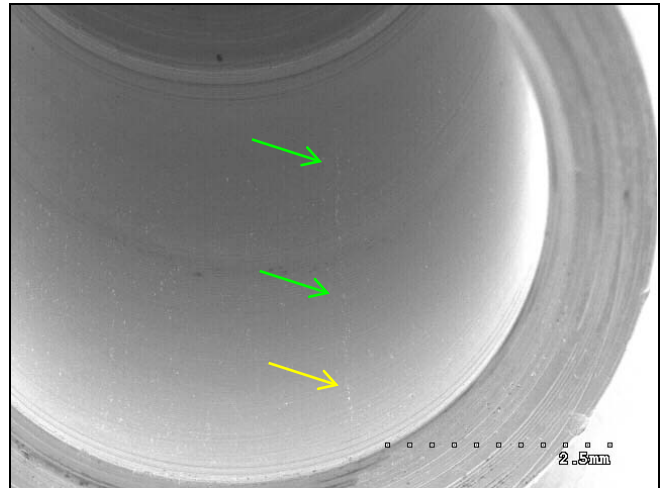
Photo 2: SEM image showing the faint linear defect indication on the machined ID surface. 10X
